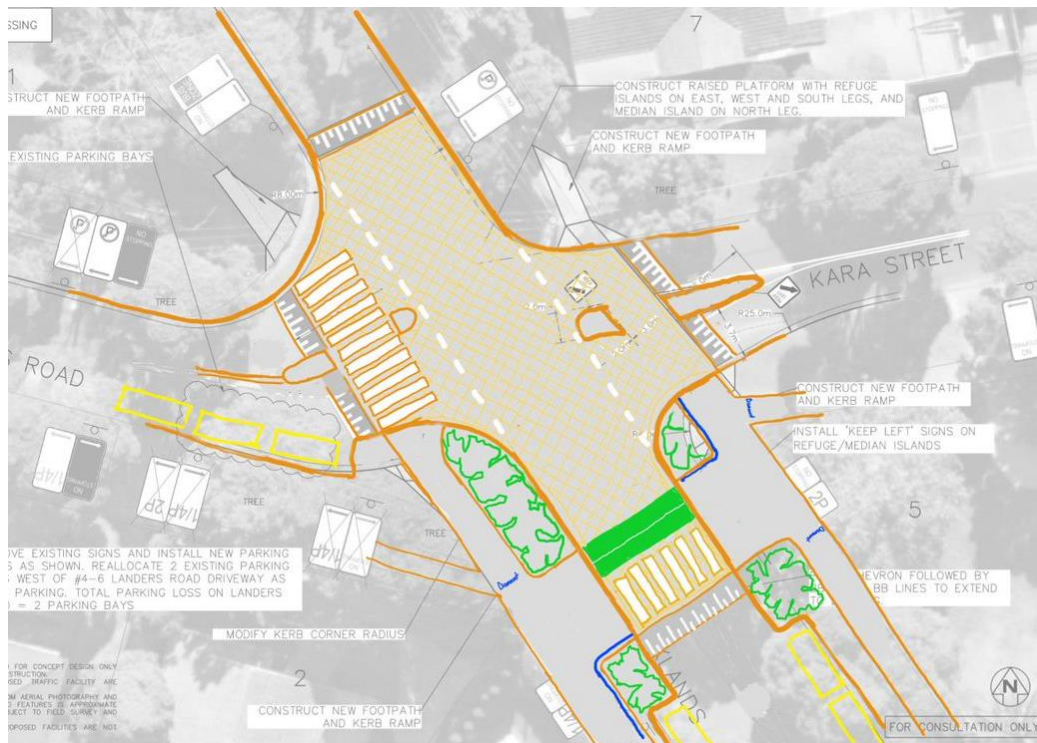
Sketch of revised layout with zebra crossings, curb extensions and shared path to Epping Road.
