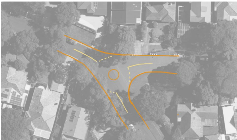
Sketch of mini roundabout layout at Parklands Avenue/Nunda Street to facilitate safe U-turns
